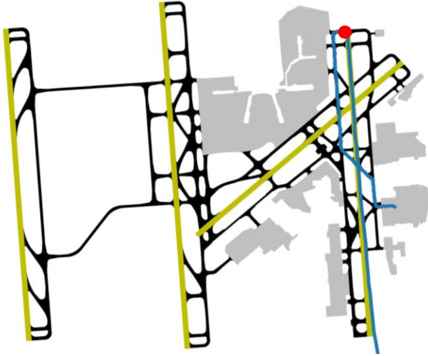
Figure 4.15 – Example of Defining Enter Runway Point (Red Dot) for Flight Path Crosses Operational Runway
