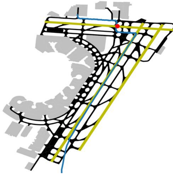
Figure 4.13 – Wrong Runway Assignment Example Based Only on Having Few Points on Runway
